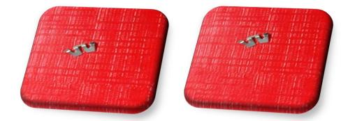
Due to this clip adapter the tool gets damage because while using the tool due to air pressure and vibration the clip adapter broke down in to small pieces and get inside the tool and damages the internal parts of the tool.
