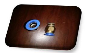
Note: If these kind of pu-pipe connector is used in the tool then it will surely damage the internal parts of tool because inside this type of connector it has clip type of pu-pipe adapter as shown below. If you are using this type of connector then our company will not give any warranty on it.
